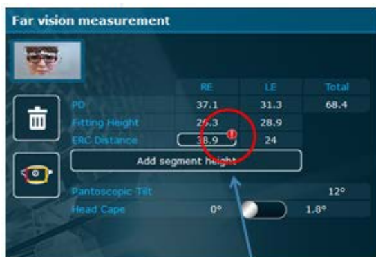
Warning sign next to the measurement
